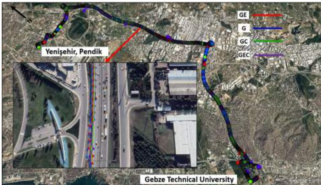
Figure 9. Display of dynamic positioning result with smartphone in Google Earth application.
